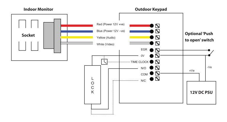
The 12V Supply is switched on to, or away from the lock by the normally open or closed terminals. The type of lock determines which terminal is used. Fail secure (N/O) Fail safe (N/C).
